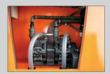
Logically designed liquid system with diaphragm pump.
