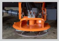
Combined disc and drop spreader with a spreading width of 1.5–6.0 m via the spreading disc. With a roller, a spreading with of 1.2 m (TP3) and 1.8 m (TP9) is achieved.
