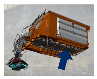
Since only the conveyor belt and material are weighed, the measurement is very accurate.
