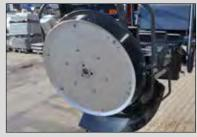
The spreading disc with or without a mixing chamber is selected independently of the spreading material.
