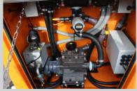
Easily accessible engine compartment protects hydraulics, control and diaphragm pump.
