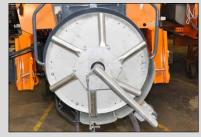
High-speed spreading using Spreading Disc. Efficient spreading at speeds of up to 60 km/h.
