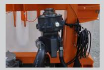
PTO operation with hydraulic pump mounted on the spreader.
