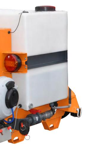
VIRTUS BASIC is designed for smaller carrying vehicles with a 3-point hitch. The machine is driven by the carrier vehicle's hydraulic system or by a PTO pump. The carrying vehicle's Tacho signal ensures liquid dosing that is dependant of road speed. The spreader boom is height-adjustable using the carrying vehicle's hitch. The spreading liquid is applied on the roadway from a low height.
