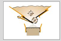
The Epoke method ensures the uniform and precise spreading of all forms of spreading material, regardless of temperature conditions or the material's characteristics.
