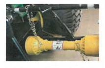
The PM 1,4 is powered by the tractor PTO and is available with 540, 800/1000 or 2000 rpm of the PTO.
