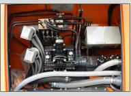
All of the vital components are located in a sealed and locked engine compartment and thus protected from salt dust. In addition, there has been increased focus on user-friendliness for the driver and service personnel.
