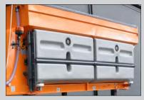
The new side tank now has a capacity of up to 3500 I (small 2200 I, medium 2592 I, large 3500 I) and has been adapted to suit the
