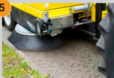
Hydraulic tilting of right side brush from remote control box
