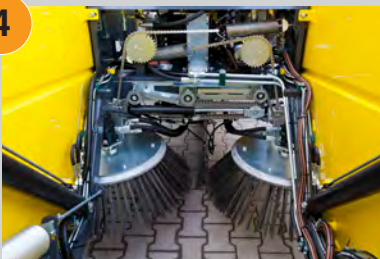
Fully automatic floating broom suspension.
