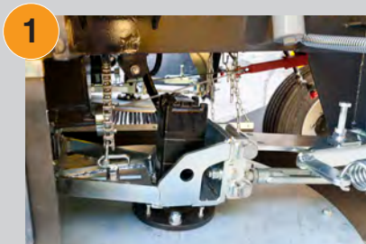
Brushes and roller adjust automatically.
