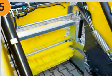
Fully automatic floating broom suspension.
