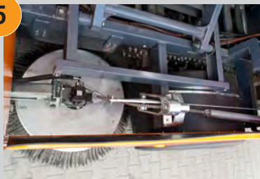
Full automatic floating brush suspension
