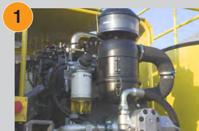
The sweeper is powered by a diesel engine - step 3 certified.
