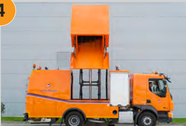
High dumping litter hopper with 3200 mm dumping height.
