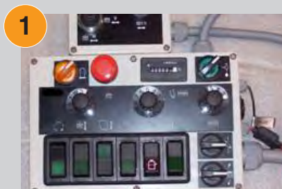
Remote control with built-in hour meter shows the operation time
