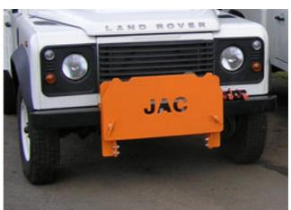
"Cubby" plate remains on the vehicle to allow the quick attachment of the snowplough.
